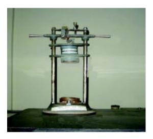
FIG. 6 : AGGREGATE IMPACT TEST MACHINE
