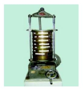
FIG. 4 : A SET OF IS SIEVES
