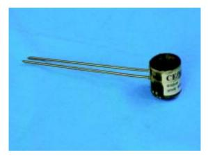
FIG. 3 : LE-CHATELIER'S TEST APPARATUS
