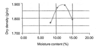
The dry density in g/cc corresponding to the maximum point on the moisture content/dry density curve should be reported as the maximum dry density to the nearest 0.01.
